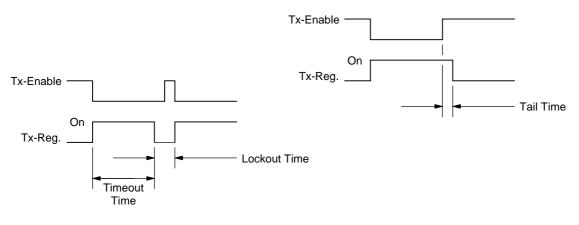
Figure 2.6 T837 Transmit Timers
