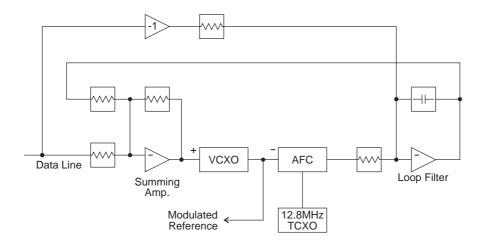
Figure 2.4 T837 AFC Block Diagram
