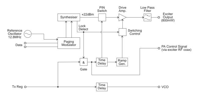
Figure 2.1 T837 High Level Block Diagram
