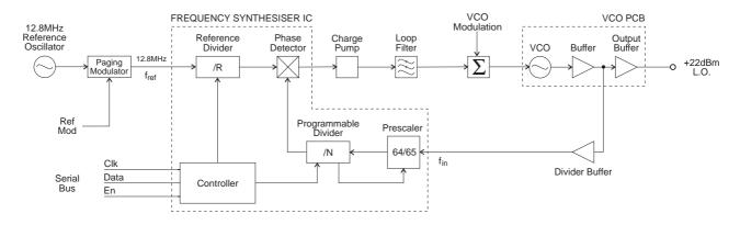
Figure 2.3 T837 Synthesiser Block Diagram
