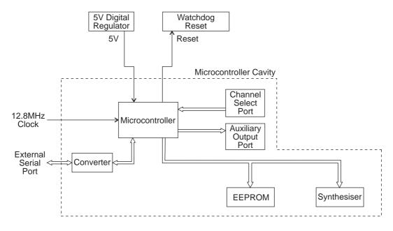
Figure 2.2 T837 Microcontroller Block Diagram
